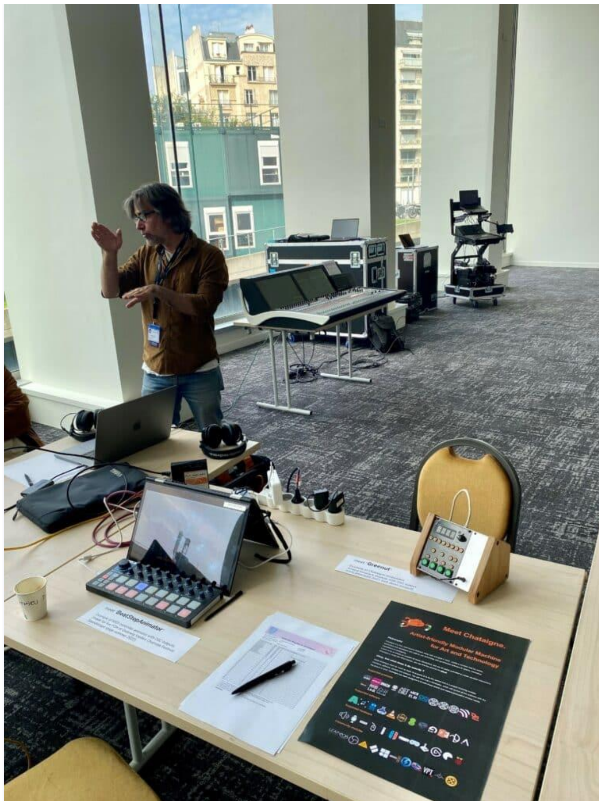
In the foreground, an example using Chataigne of a live controller using ADM-OSC https://github.com/madees/BeatStepAnimator as well as a prototype of a CV>ADM-OSC module in Eurorack format. Behind, Martin Antiphon from AES France discusses his space synthesizer and binaural rendering engine MyBeeKnows developed with Music Unit. Then, the Lawo mc236 console and its ADM-OSC plugin. Finally, in the background, Hervé Déjardin's 3D stage audio controller.
